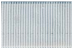
FLUITEX® E – 6 mm thick polyester fabric
