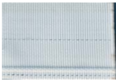
FLUITEX® E – 4 mm thick polyester fabric with breadding
