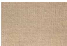
FLUITEX® AD – 4 mm thick heat resistant para aramid fabric
