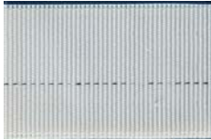
FLUITEX® E – 4 mm thick polyester fabric
